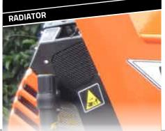
The C60 has a powerful radiator with fan and thermostat to cool the hydraulic system.
