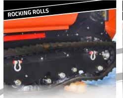
the machine's undercarriage, unique to the Cormidi line, has suspensions follow the terrain profile for increased stability and comfort.
