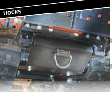
4 Large and sturdy hooks to move the machine in total safety, plus 2 for towing.
