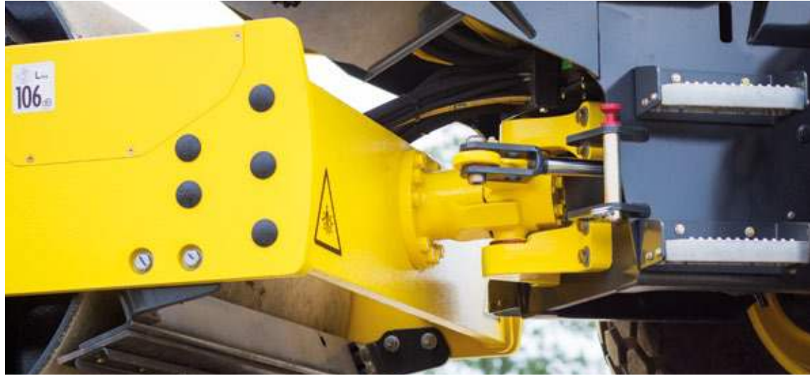
Cleanly engineered: the articulated joint is maintenance-free; the machine requires no lubrication whatsoever.
