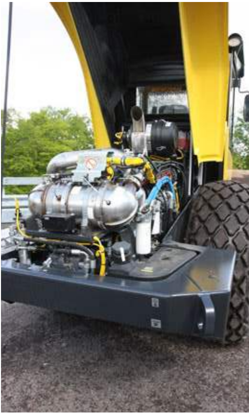
All cables protected from damage.
