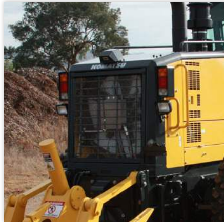
Easy radiator cleaning with reverse fan
