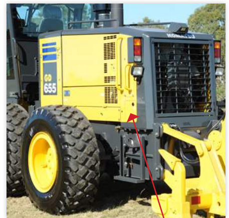
Lockable- ground level refuelling.
