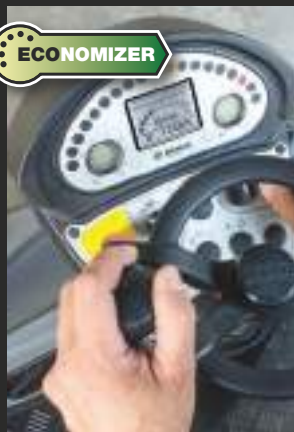
Compaction progress display.
