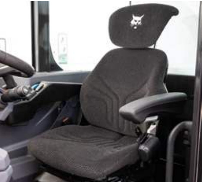
Grammer Maximo Air suspended seat with heating, Dynamic Dumping System (DDS) and joystick mounted on suspended armrest
