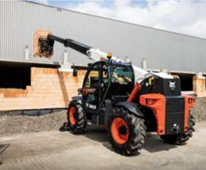
Hydrostatic transmission with dynamic mode for more agility comes as standard for all models.
