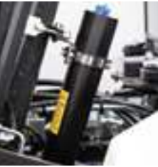
Boom suspension (Nitrogen accumulator)
