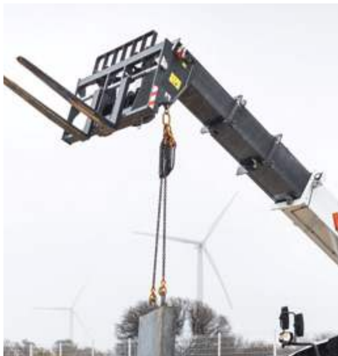
Lift eye on boom head (model depending)
