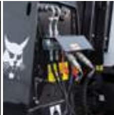
Auxiliary hydraulic line on boom head with FCS*
