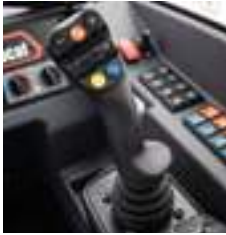
Smart joystick with Boom float and bucket shaking
