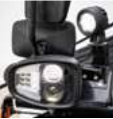
LED road pack: • road lights • rotating beacon • reversing light
